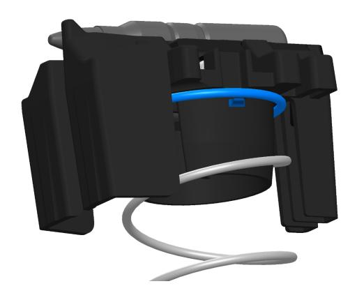
11. Insert the follower assembly into the magazine body QTR0016. Verify the follower is oriented correctly with the body and that the grooves are in line as shown.
