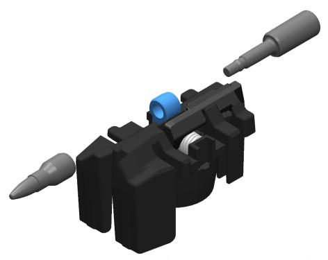
6. Insert the tail QTR0013 into the link. Verify the tail is oriented to the back of the follower as shown.
