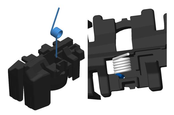
2. Hook the lifter QTR0015 into the corresponding cut out in the follower and place the other leg of the spring HDW0106 in the groove of the cut out. The spring will be semi compress and will need to be guide.
