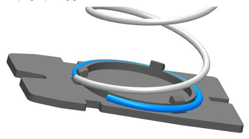
10. Attach other end of the spring to the follower assembly by applying pressure and rotating the spring. Verify that three prongs are engaged.
