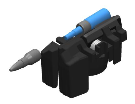
7. Insert the head QTR0014 onto the tail and apply pressure until the head fully engages the tail and link.
