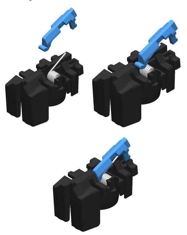
3. Push down on the riser QTR0015 until the leg of the riser engages the follower and verify the the riser moves completely down with no resistance once engaged. It is important that the spring is not bound to ensure proper functionality.
