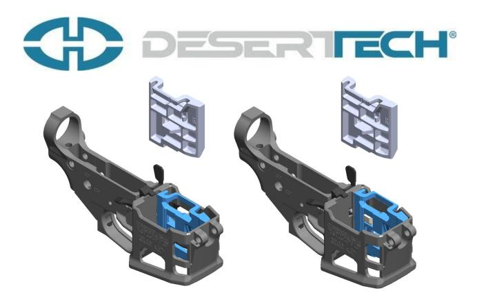
17. Press firmly of the insert until the clip engages the outside of the reciever as shown.
