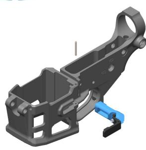
3. Insert QTR0001 partially into magazine button cut of QTR0004 until the spring QTR0006 meets the edge of the cut.
