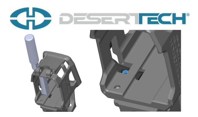
5. Push the button the rest of the way and verify the spring is oriented correctly.
