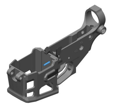
13. Drive the pin .100" down below top surface with a 5/32" dia 6" long driver from the front of the receiver. (a 3/32" dia driver is required to remove the pin)
