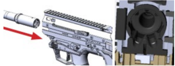
Figure 43: Installing Barrel Assembly
